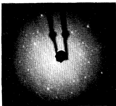
Figure 5. Diffraction pattern from the stable form of the Si(111) surface which exhibits (7 \times 7) structure.
